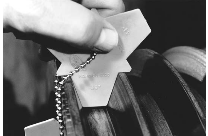
Pulley gauges make wear detection easier.
